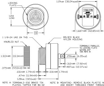
NOTE A: TERMINALS-0.32 BRASS TIN PLATED, TAPPED FOR #6-32 SCREW. TWD #6-32 NICKEL PLATED BRASS SCREWS INCLUBED. WILL ACCEPT 1/4' QUICK CONNECT. NOTE B: MOUNTING- REMOVE BLACK PLASTIC NUT AND INSERT THREADED FRONT THROUGH 1.25' HOLE PUNCHED IN PANEL, IF DRIENTATION IS NEEDED, NOTE LOCKING FLATS ON DRAVING. SCREW NUT BACK ON. DO NOT OVERTIGHTEN.
